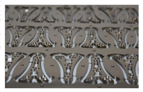
Task definition De-burring and rounding of the milled contours
